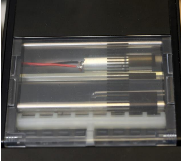
Normal tape position – diverter in CLOSED position
